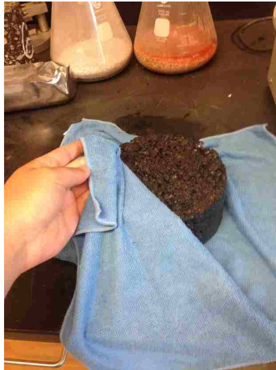
Figure 3.5 Bulk specific gravity procedure
