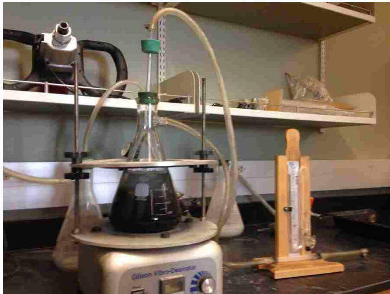
Figure 3.3 Maximum theoretical specific gravity procedure
